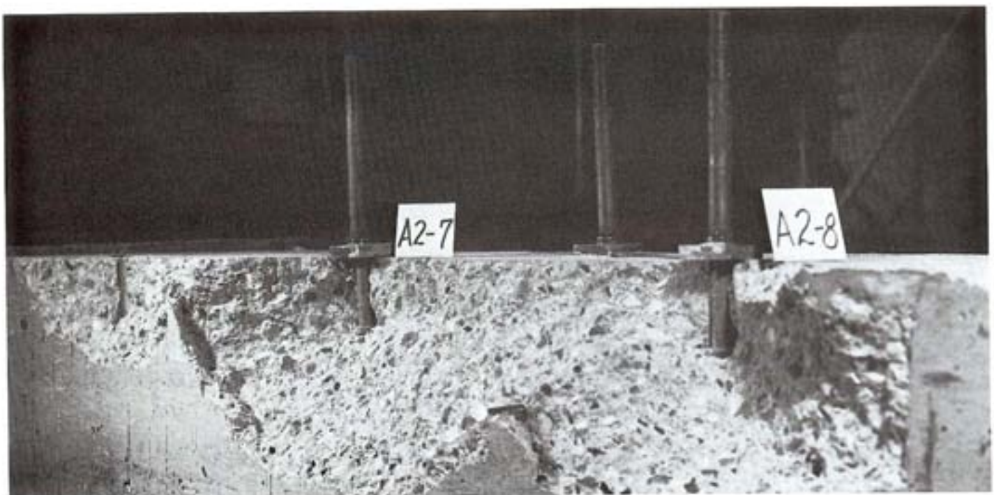
FIGURE 21.—Specimens A2-7 and A2-8 (3) , \frac{3}{4} \times 4\frac{3}{16} " Anchors, Subject to Pure Shear, 6" From Free Edge.
