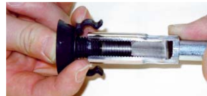
Screw the nailing plate into the data clip to drive the HSS protector down the socket. Rotate the data clip in the desired direction (depending on the position of the angled lift reinforcement).
