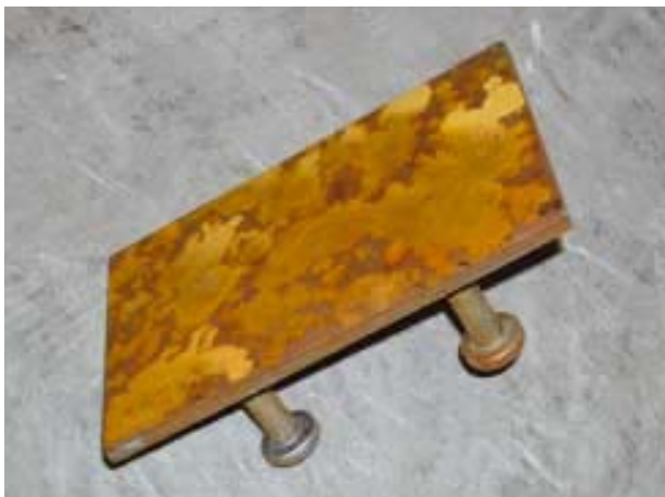
Welded connections require painting to give minimal corrosion protection.
